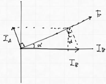
$$\sin \alpha = \frac{I_B \omega L - I_B \frac{1}{\omega C_B}}{E} = \frac{I_A}{I_B}$$
