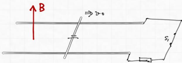
$$(1) \Delta \bar{\Phi} = B l v_0 t$$
