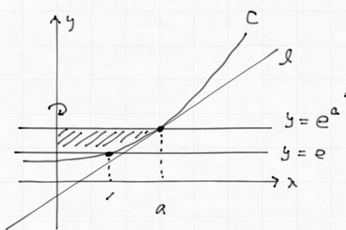
$$\begin{aligned} V &= \int_e^{e^{a^2}} \pi x^2 dy \\ &= \int_1^a \pi x^2 \cdot 2x e^{x^2} dx \\ x^2 = t \text{ とおく } \quad \left( \frac{dt}{dx} = 2x \right. &\left. \frac{x}{t} \Big|_{1 \rightarrow a^2} \right) \end{aligned}$$
