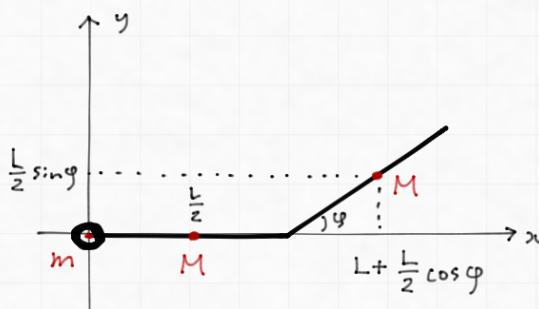
$$\begin{pmatrix} x_G \\ y_G \end{pmatrix} = \frac{m}{m+2M} \begin{pmatrix} 0 \\ 0 \end{pmatrix} + \frac{M}{m+2M} \begin{pmatrix} \frac{L}{2} \\ 0 \end{pmatrix} + \frac{M}{m+2M} \begin{pmatrix} L + \frac{L}{2} \cos \varphi \\ \frac{L}{2} \sin \varphi \end{pmatrix}$$
