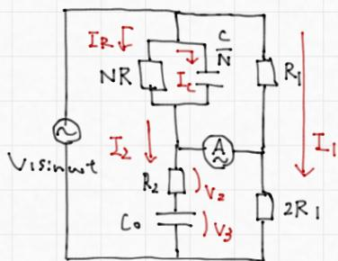
$$V_{K-M} = \frac{2R_1}{2R_1+R_1} V_1 \sin \omega t = \frac{2}{3} V_1 \sin \omega t$$
