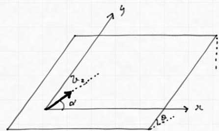
$$\begin{aligned} & \text{2 cases consider} \\ & \text{case 1 } \tan\alpha = \frac{1}{2} g \sin\theta \cdot \frac{x}{v_0^2 \cos^2\alpha} \end{aligned}$$
