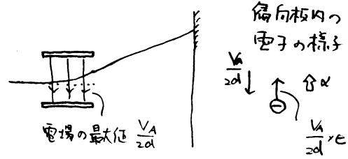
$$\lambda_M = \frac{hc}{e(V_0 + \frac{V_H}{2})} = \frac{2hc}{2e(V_0 + \frac{d^2 V_0}{\lambda^2})} = \frac{hc \lambda^2}{eV_0(\lambda^2 + 4d^2)}$$
