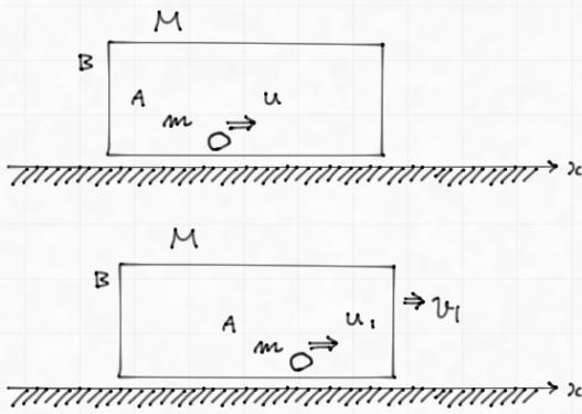
$$\text{小球Aの運動量の変化} = mu_1 - mu = \text{力積} = \bar{f}_{\Delta t} \quad (1)$$
